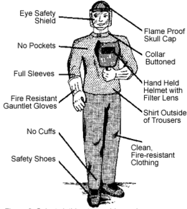
Figure 3. Select clothing to provide maximum protection from sparks and hot metals
